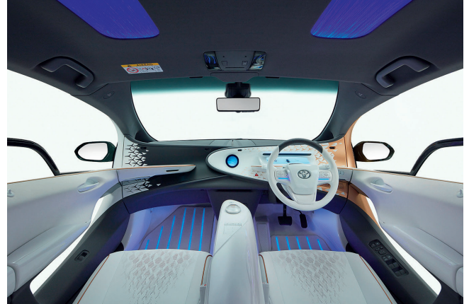
Fig. 5. A PU from Covestro reinforced with Kenaf fibers was used in the door panel of the "LQ" concept vehicle. As such, it is 30% lighter than the previous models © Toyota
