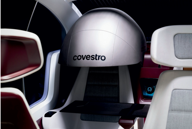
Fig. 4. The Baynat PU system from Covestro provides effective sound insulation in the PrivacyDome, an extendable dome. Noise production plays a vital role for electrical and autonomous driving vehicles © Covestro
